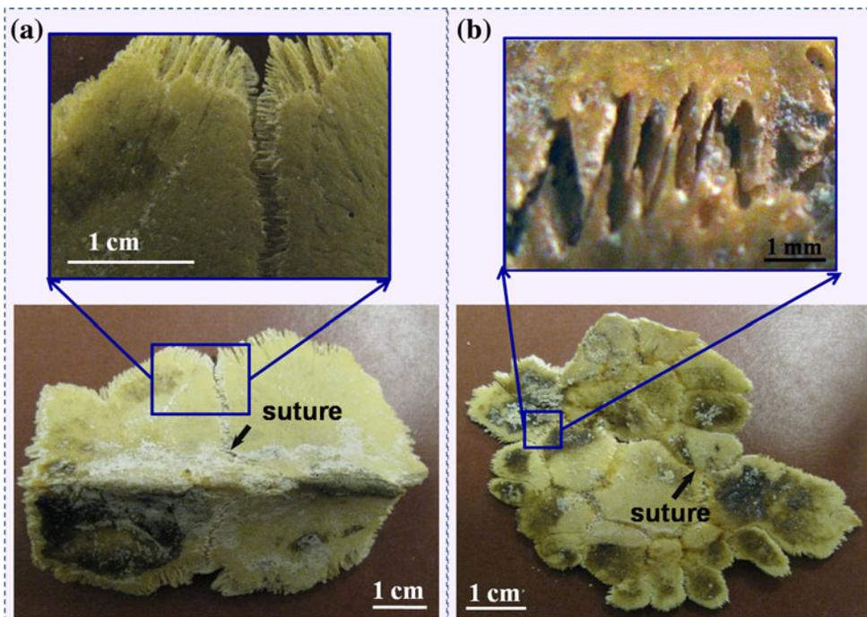
Fig. 4. Leatherback turtle plates: (a) two juxtaposed plates from a dorsal ridge and (b) from plastron. Note the irregular-shaped sutures that act as a junction between plates.
