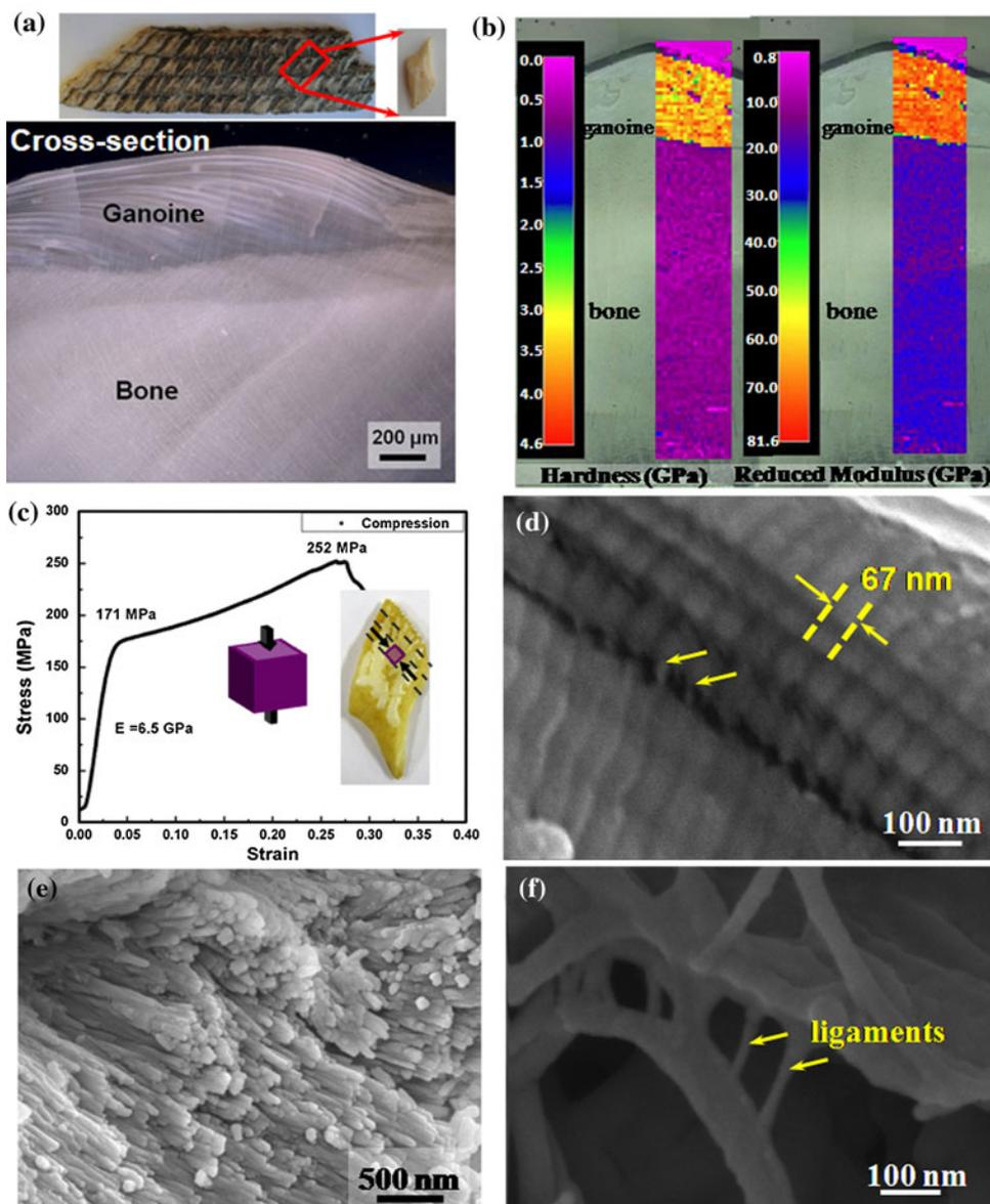
Fig. 5. Structural details and mechanical performance of alligator gar scales: (a) scales and cross section; (b) nanoindentation hardness and reduced modulus through the thickness of the scale; (c) compressive stress strain curve for bone portion (d) mineralized collagen fibers; (e) HAP crystals; and (f) ligaments between collagen fibrils.
