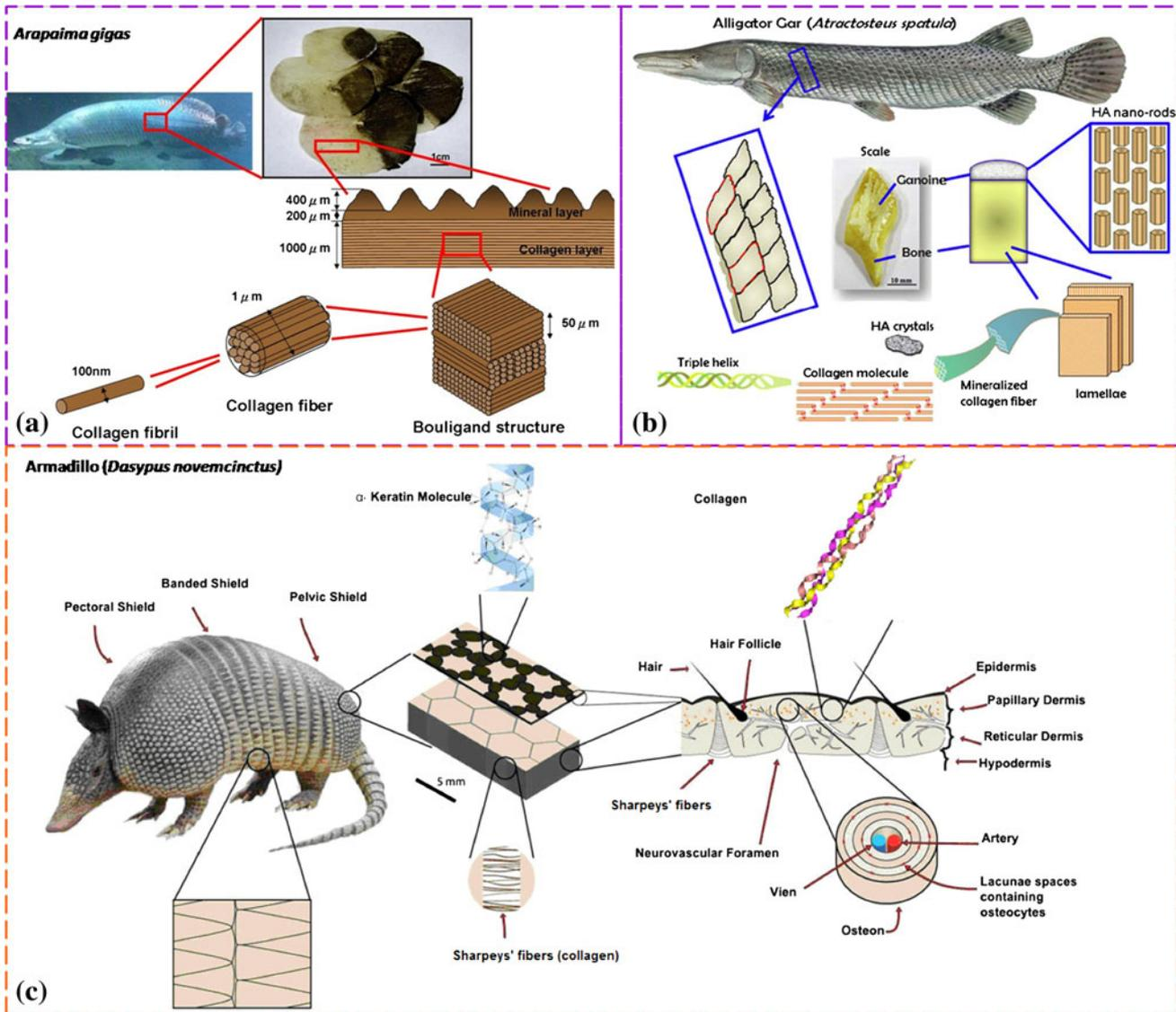
Fig. 2. Hierarchical structure of three flexible dermal armors: (a) arapaima,<sup>7</sup> (b) alligator gar,<sup>7</sup> and (c) armadillo.<sup>12</sup>
