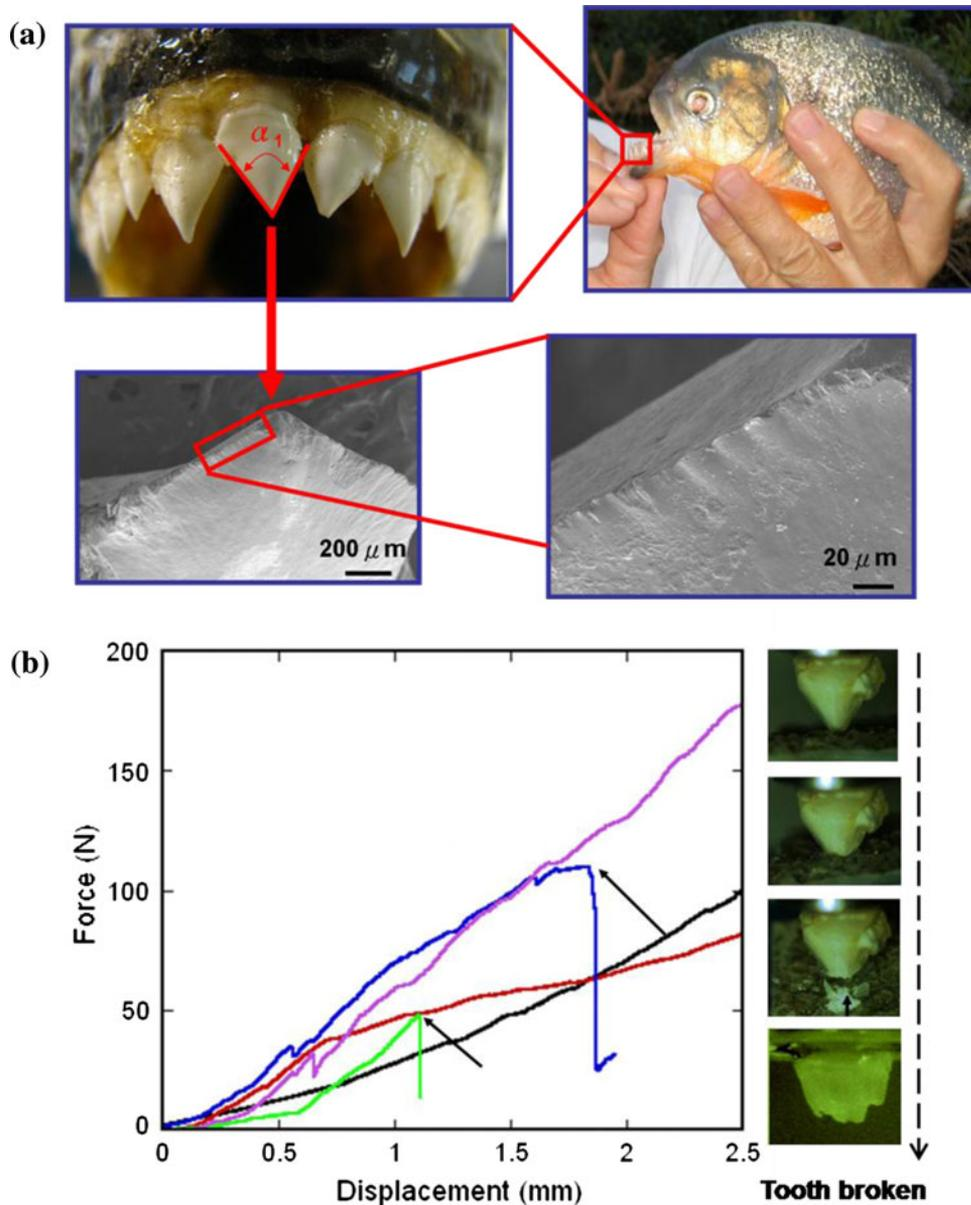
Fig. 9. Piranha teeth and their puncturing effect on arapaima scale: (a) red piranha and details of teeth; and (b) force-penetration by piranha tooth through external region of arapaima scale. Note that load drops corresponding to fracture of teeth before full penetration (2 mm) is accomplished. Tooth penetration and fracture shown in right-hand side.<sup>17</sup>
